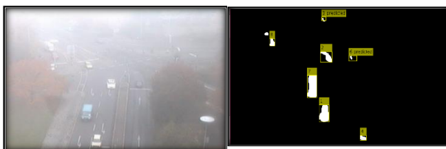
Fig1 Segmentation object at 65 frame per second from Karlsruhe Data Set in fog environment.
